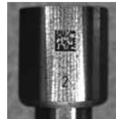
Figure 10: Laser-marked code on a metal cylinder
